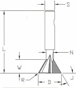
D= \_\_\_\_\_ DOVETAIL DIAMETER
